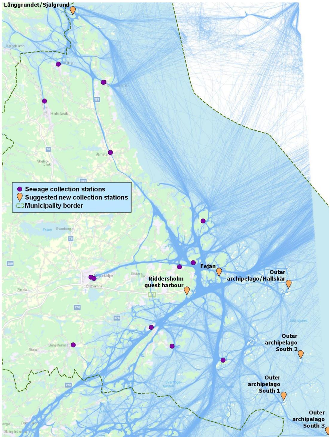
Figure 1. Existing collection points for sewage from small boats (purple dots) and suggestions for localization of new sewage collection points (orange tear-shaped markers). Blue lines represent boat movements recorded from AIS-transponders during the summer of 2018.
